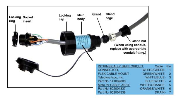
Figure 2-13 Network cable connector and wiring
